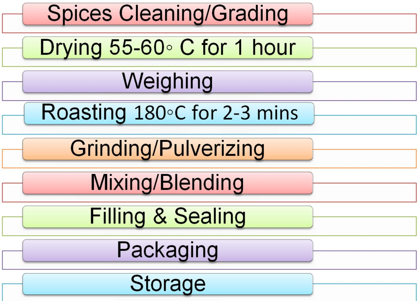
The process of manufacture involves cleaning, drying, pulverizing, sieving and packaging of spices such as chilli, pepper, turmeric, coriander, etc. either individually or in combination with other spices. There are various formulations for curry powder, but the ingredients like red chilli, black pepper, cloves, coriander seed, cumin seed,
