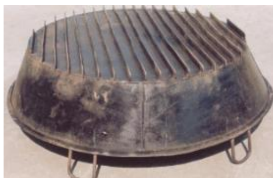
Modified pans for jaggery furnace
