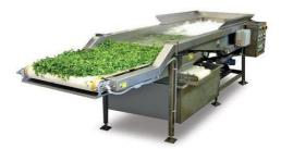
**Blancher:** This machine is used for blanching operations to inactivate enzymatic activities and destroy microorganism.
