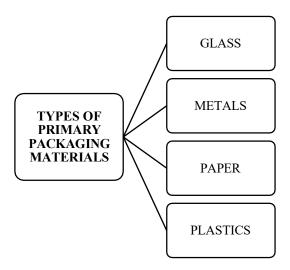
**GLASS**-Glass possesses very good barrier properties, so it maintains product freshness for a long period of time without impairing the taste or flavor, visibility of product, the ability to withstand high processing temperatures.
