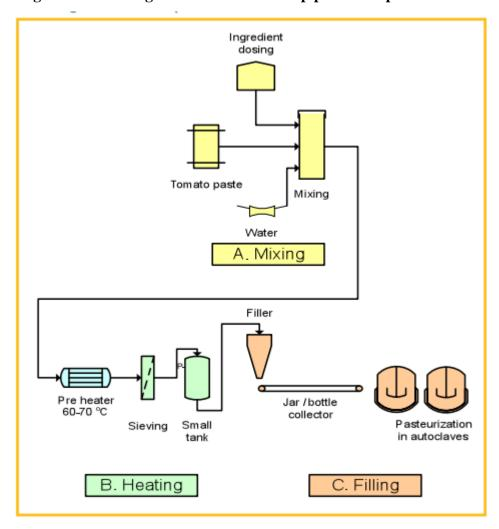
Figure 4: Flow diagram of tomato ketchup process at pilot scale level
